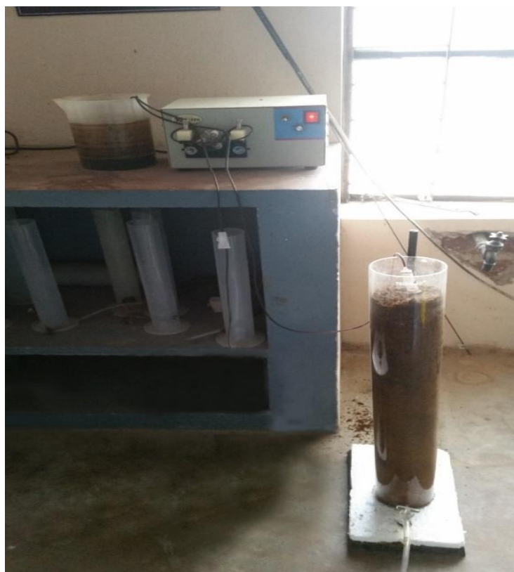
Figure 2: Experimental setup of 60 cm rice husk packed bed column
